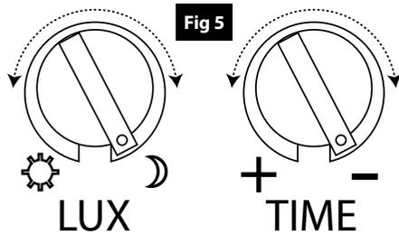
**ADJUSTING THE DURATION TIME:** the length of time that remains switched on after activation can be adjusted from (10±5) seconds to (4±1) minutes; rotating the TIME knob from (+) to (-) will reduce the duration time.
