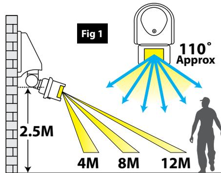
To avoid damage to the unit do not aim sensor towards sun.
