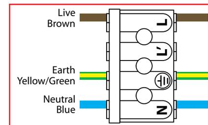
Terminal capacity: 0.5mm<sup>2</sup> - 2.5mm<sup>2</sup>
