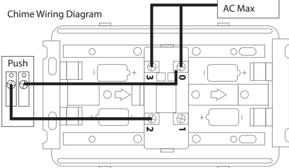
**NOTE:** Please use a transformer unit when using with an illuminated bell push, as the light will drain the batteries.
