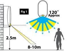
To avoid damage to the unit do not aim sensor towards the sun.
