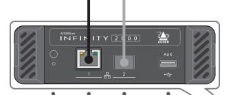
Status indicator and reset network port USB switch Primary (SFP) port
