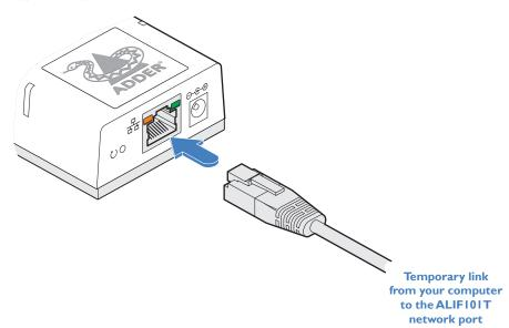
2 Connect the other end of the link cable directly to the network port of your computer.
