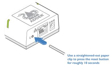
3 Release the reset switch at the appropriate time (see the table above).
