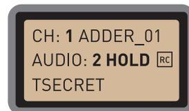
The status display also shows the current channel number; the channel from which audio is being derived and also the remote control unit status.
