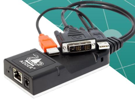
**High Performance ZeroU™ IP KVM dongle for extension or matrix of video, audio and USB over a single cable**
