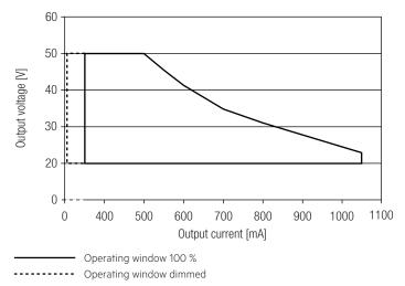
Make sure that the LED Driver is operated within the given window under all operating conditions. Special attention needs to be paid at dimming and DC emergency operation as the forward voltage of the connected LED modules varies with the dimming level, due to the implemented amplitude dimming technology. Coming below the specified minimum output voltage of the LED Driver may cause the device to shut-down.
