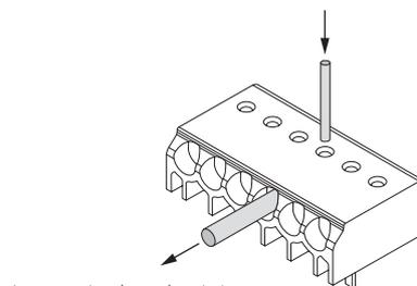
Loosen wire through twisting and pulling or using a Ø 1 mm release tool
