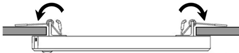
(Surface Mounting) Step 1: Twist and remove the bracket from the fitting. Remove the extension springs from the bracket.
