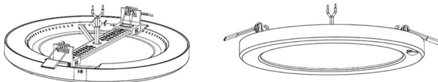
(Recess Mounting) Step 2: Before cutting, ensure that the hole does not impinge on joists, pipe work, cables or other building services.
