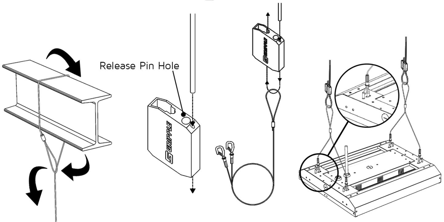
Step 1: Wrap Anchor Wire around mounting beam, then feed loose end through the wire loop and pull on the loose end to secure.
