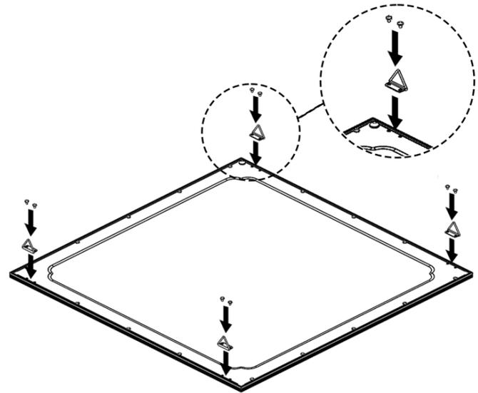
Step 5: Align brackets with the corner fixing holes, then attached the 2x securing screws in each corner. Use longer securing screws supplied with kit.
