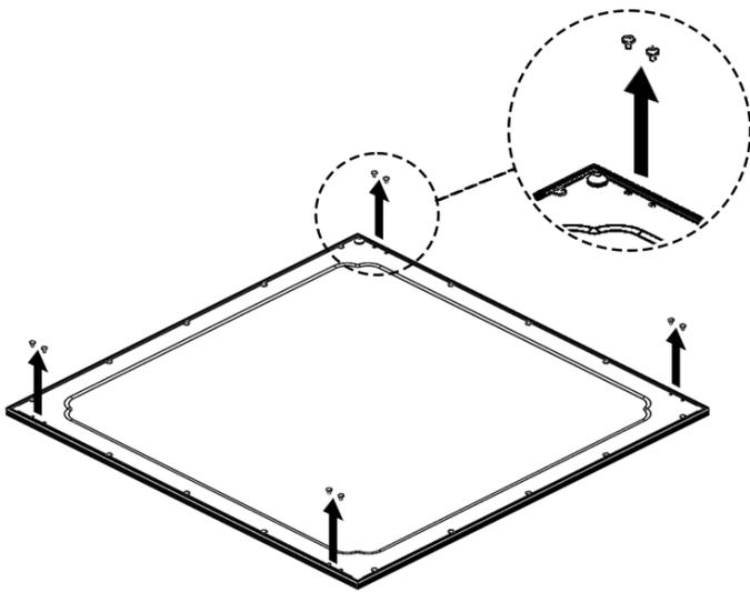
Step 4: Remove 2x rear securing screws from each corner.
