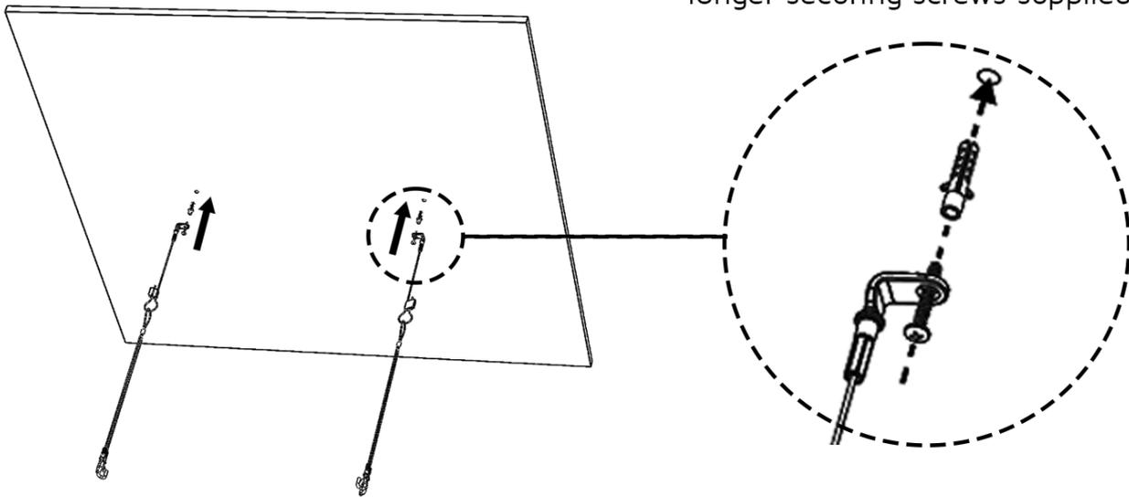
Step 6: Attach the Anchor Wires to the ceiling with suitable rawl plugs and fixing screws.
