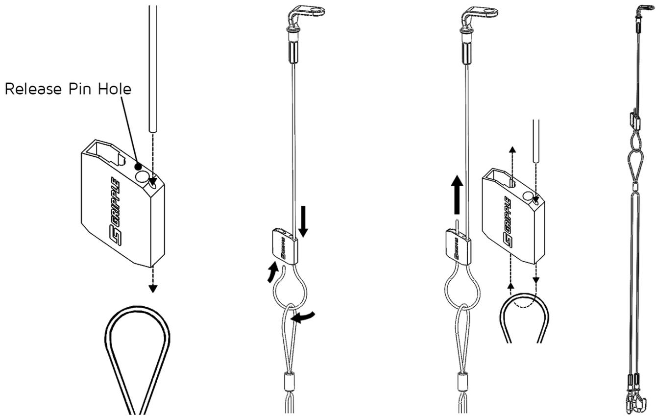
Step 1: Feed Anchor Wire into the Metal Clasp
