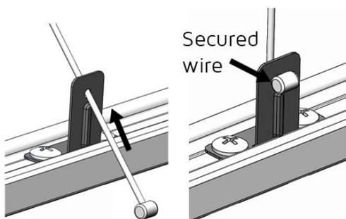
**Step 3:** Attach suspension wire to top fixing bracket, then secure to ceiling.
