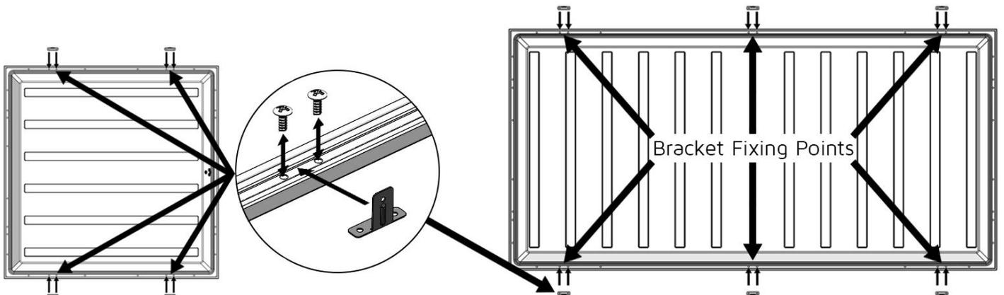
**Step 2:** Insert suspension wire into bracket and pull through until secured against bracket.
