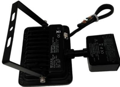
**Step 4:** Remove the waterproof cover on the bottom of the motion/photocell sensor. Configure the switches to set the desired functions using the table below.
