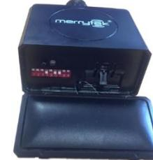
Default settings are: Detection Area 100%, Hold Time 1min, Daylight Sensor operates at 50Lux, Motion Sensor on.
