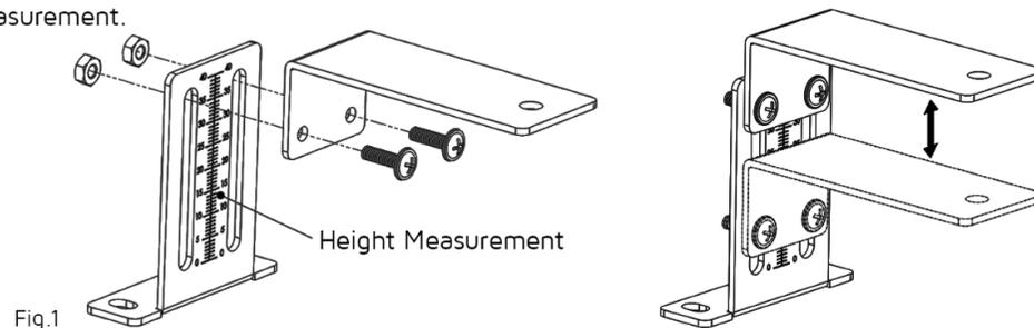
Step 3: Remove the 2x Panel screws in each corner of the LED Panel. Align the Bracket with the panel holes, then insert the 2x panel screws to secure the bracket.
