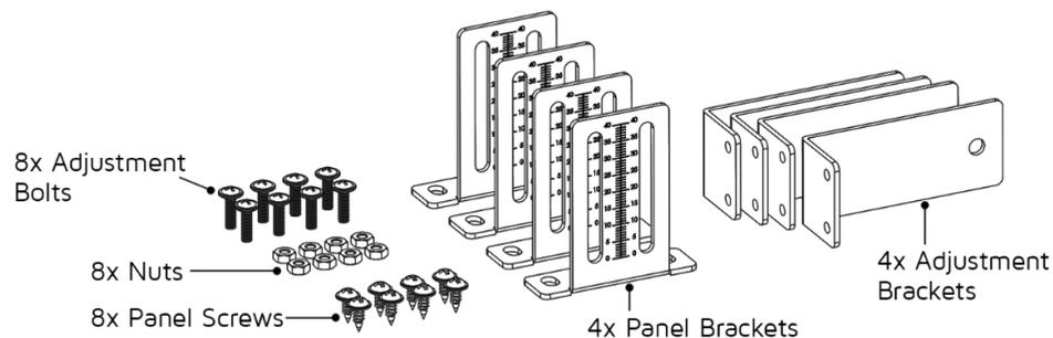
Step 2: Assemble the Z Bracket as per Fig.1 shown below. Adjust the height of the bracket according to the thickness of the ceiling. Ensure that all 4x brackets are set to the same height measurement.
