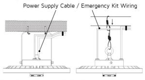
Note: Do not tamper with the Emergency kit wiring unless installing an Emergency Kit (High Voltage).
