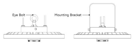
Mounting Bracket installation: Attach the mounting bracket to the High Bay with the 2x M6 Anchor Bolts. Adjust the angle of the bracket, then attached the 2x securing screws.
