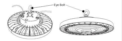
Step 2: Mount the High Bay light to the ceiling using a chain or a suitable suspension kit.
