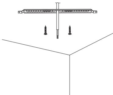
Knock-in the plastic anchor into ceiling, fix bracket with screw.
