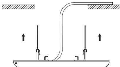
Hold back the spring clip then push the downlight into the hole.
