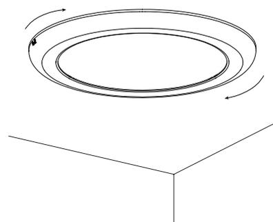
Aim the groove at the installation bracket, rotate the lamp clockwise until it is firmly fixed, turn on.
