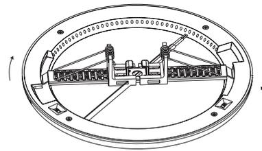
Rotate the bracket clockwise until it fix tightly with lamp groove.
