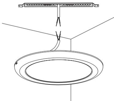
Connect wires with L,N, and do insulation treatment.
