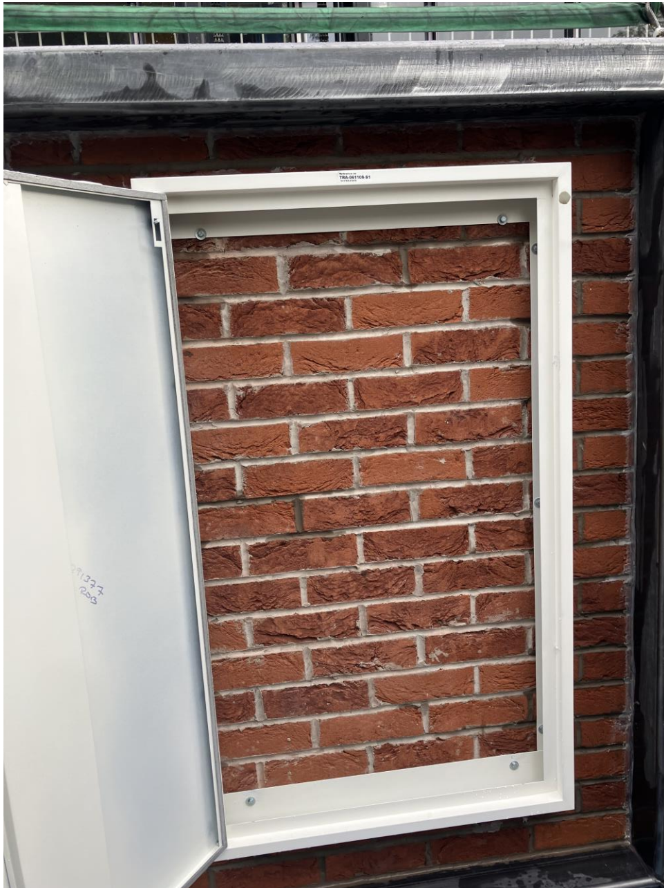
Specimen Test Configuration for Ingress Protection Tests
