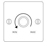
Rotate the knob to program the minimum brightness levels.
