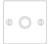
When the lamp is switched **ON**, press and hold "**PUSH KNOB**" for 3-5 sec until the lamps appear at half their brightness level.
