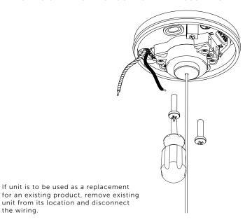
CONNECT THE WIRES AS SHOWN IN APPROPRIATE WIRING DIAGRAMS. USE GREEN/YELLOW SLEEVING ON EARTH CONDUCTORS THAT ARE NOT INSULATED. ENSURE TERMINALS ARE PROPERLY TIGHTENED AND NO BARE WIRE IS VISIBLE. PUSH BACK UNIT INTO MOULDING BOX MAKING SURE CONDUCTORS ARE NOT TRAPPED.
