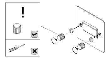
\*\* Do NOT use a standard screw driver to tighten the coin caps. This may damage the cap and is not covered under warranty. Plastic coin cap tool must be used by hand only.
