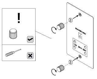
\*\* Do NOT use a standard screw driver to tighten the coin caps. This may damage the cap and is not covered under warranty. Plastic coin cap tool must be used by hand only.
