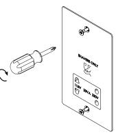
\* Please ensure screws are sufficiently tight to support the product but please do not over tighten as this may cause some deformation to the plate or damage the screw.
