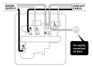
\* This fused connection unit is fitted with two linked terminals to provide a dual earth facility. This is for use in "clean earth" installations were additional earth capacity is required to comply with regulation 607 of BS 7671 IET wiring regulations.
