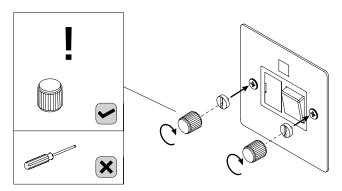
\*\* Do NOT use a standard screw driver to tighten the coin caps. This may damage the cap and is not covered under warranty. Plastic coin cap tool must be used by hand only.
