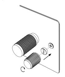
\* Please ensure screws are sufficiently tight to support the product but please do not over tighten as this may cause some deformation to the plate or damage the screw. \*\* Do NOT use a standard screw driver to tighten the coin caps. This may damage the cap and is not covered under warranty. Plastic coin cap tool must be used by hand only.
