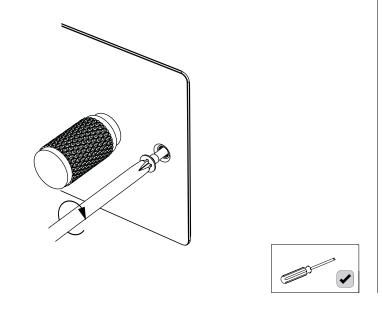
**4C.** By hand, screw the coin caps into the end of the screws. Use the plastic coin cap tool to fully tighten the coin caps\*\*.
