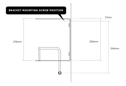
CERTAIN ITEMS IN THE RANGE WILL NOT FIT INTO A 4 LUG BOX. IF SUCH A BOX HAS BEEN PREVIOUSLY INSTALLED THE TOP AND BOTTOM LUGS SHOULD BE REMOVED OR BENT BACK TO AVOID CONTACT WITH THE INTERIOR.
