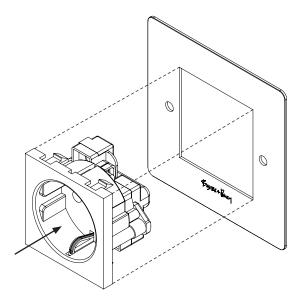
ONCE MODULE IS SECURELY IN PLACE — USE A CROSS HEAD ELECTRIC OR MANUAL SCREWDRIVER TO FIT THE COUNTERSUNK SCREWS UNTIL TIGHT\*.
