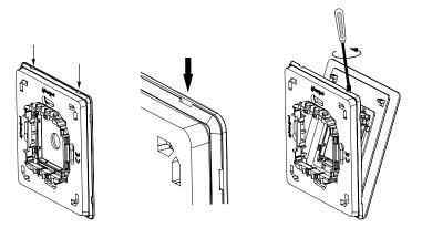
Snap-in the dimmer to the plate before screwing the container to the wall
