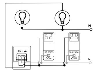
The Dimmer must always be connected to the LINE side of the load. You can have up to 20 retractive switch or push switch connected to your dimmer to control from multiple locations.
