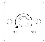
Rotate the knob to program the minimum brightness levels.
