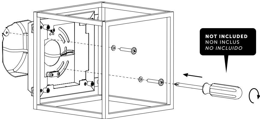
**EN:** Wall fixings not included. Fixings used should be suitable for the intended location and weight of the product.
